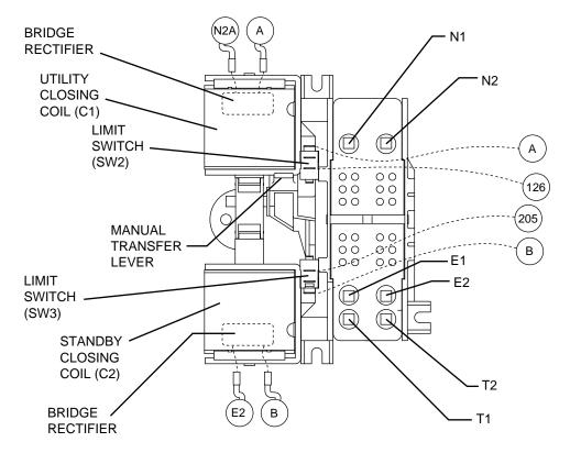
Figure 1. The Transfer Mechanism
